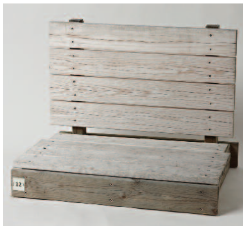
Tanalised Clear treated 2 year exposure
