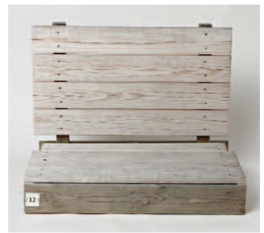
Tanalised Clear treated 2 year exposure
