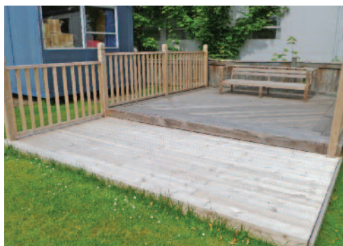
Castleford test deck - 10 months exposure, June 2011
